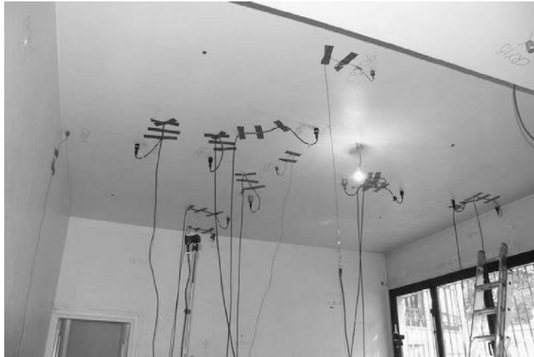
Fig. 5. The measurement site in the basement with accelerometers on the ceiling.
